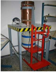
I. Shielded Ge-(HP) detector for gamma and X-ray
