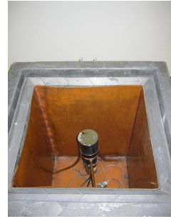
II. Scintillator detector NaI(Tl) for gamma radiation
