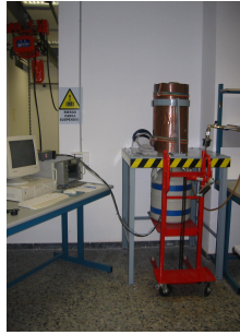
I. Shielded Ge-(HP) detector for gamma and X-ray
